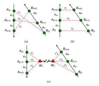
Fig. 1. Neighbor discovery scenarios for two nodes A and B with solid lines showing movement, dashed lines indicating connectivity, and  $W_1$  and  $W_2$  representing the ends of a wormhole. a) Two mobile nodes move in opposite directions. b) Two mobile nodes move in the same direction. c) Two mobile nodes communicate through a wormhole. The range perceived by nodes is  $r_i = r'_i + r''_i$ .
