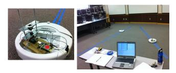
Fig. 5. Experimental evaluation using Epic motes ranging with SRF-02 ultrasonic range finders and carried by iRobots. A mobile node equipped with ranging hardware, and experimental setup.
