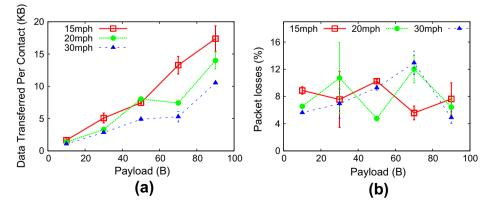
Fig. 14. Zigbee contact performance - (a) data transferred per contact and (b) packet loss per contact.
