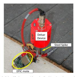
Fig. 2. Delsar life detector with steel spike driven into the ground, and interfaced with an EPIC mote.
