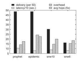
**Fig. 16.** Evaluation of latency, delivery rate, overhead and average hop count for four different DTN routing protocols in simulation.
