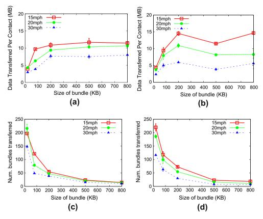
Fig. 13. Per-contact performance for WiFi: the DTC without security (a) and with security (b); the number of bundles transferred without security (c) and with security (d).
