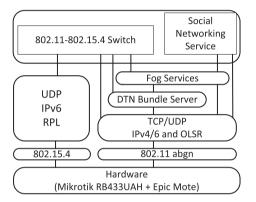
Fig. 6. DistressNet software architecture: Class C: Network backbone.
