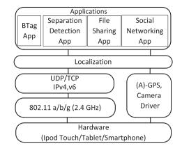
Fig. 5. DistressNet software architecture: Class B: End user interactive.
