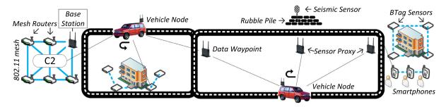
Fig. 1. Schematic of a DistressNet deployment showing all components. Data generated by BTag and Seismic Sensors is ferried to the Base Station using Vehicle Nodes. A Data Waypoint improves the data transfer process by creating a contact opportunity between two Vehicle Nodes.
