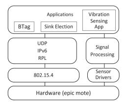
Fig. 4. DistressNet software architecture: Class A: Sensing.
